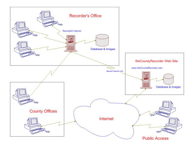
theCountyRecorder™ is designed in a client server architecture.
